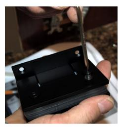
6. Open the box of hinges and remove one hinge from the protective bag. Unscrew the two hex bolts holding the hinge plate to the hinge, using the hex key provided. Take care not to scratch the hinge or bolts.
